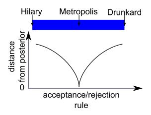
Only the Metropolis accept/reject rule allows sampling from each point in exact proportion to the posterior height.
